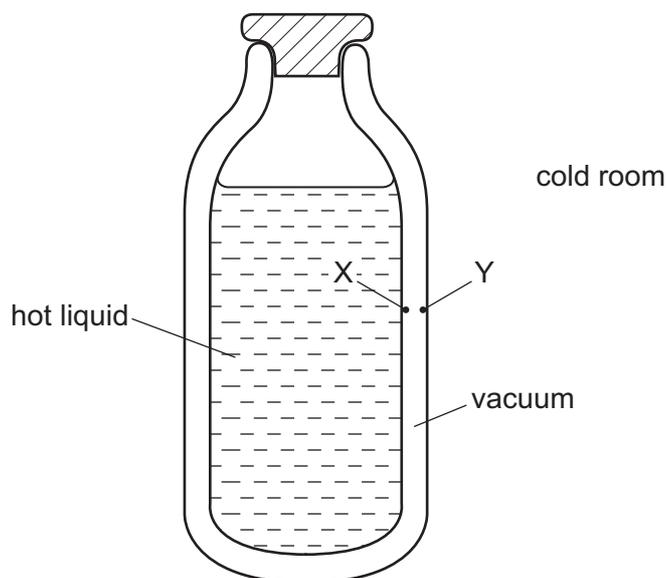
How is thermal energy transferred through the vacuum between X and Y?
